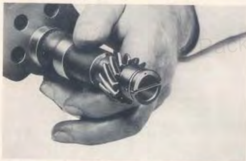
Fig. 50—Showing Position of Drive Gear Prior to Installing Pump on Eight Cylinder Engine. Note Punch Mark.
