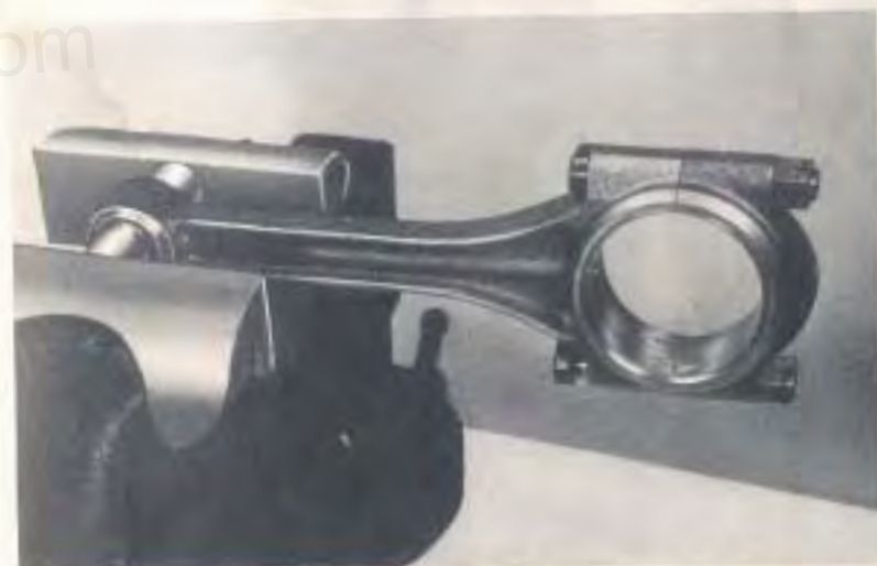
Fig. 21—The Connecting Rod Should Remain in a Horizontal Position Until Tapped Downward by Hand.
