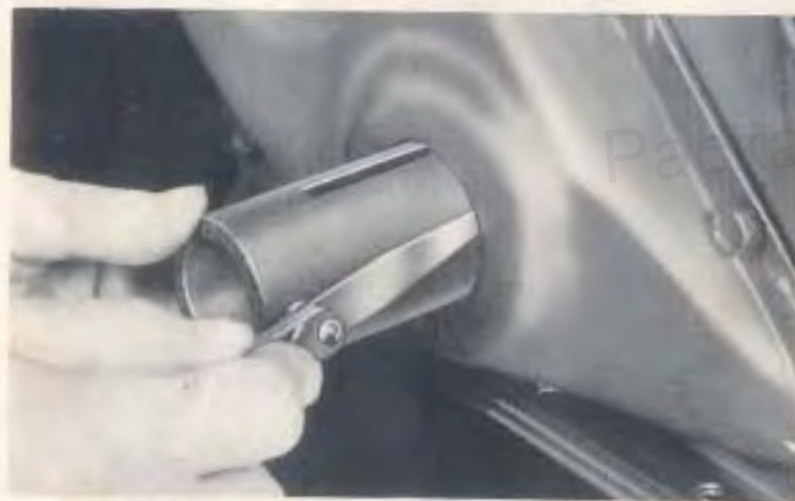
Fig. 33—The Gear Cover Should Be Shifted to Obtain the Same Clearance Around all Sides of the Arbor.
