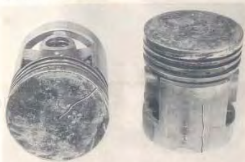
Fig. 9—Pistons Should Be Closely Inspected After Cleaning. Note the Cracks in the Piston Head and the Skirt.
