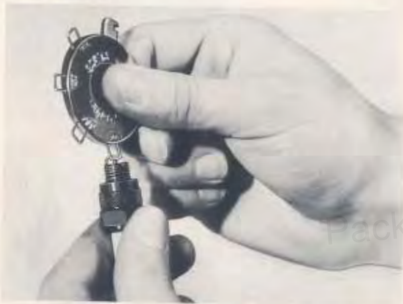
Fig. 53—The Spark Plug Gap Should Be Checked with a Round Wire Gauge Tool.
