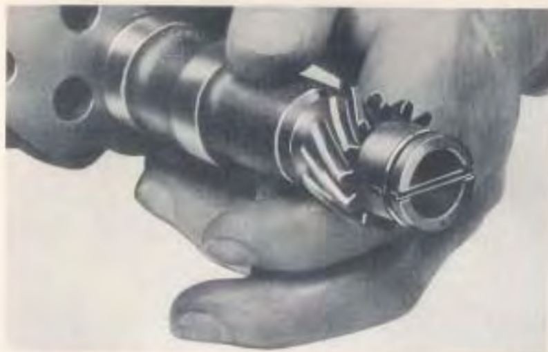
Fig. 49—Showing Position of Drive Gear Prior to Installing Oil Pump on Six Cylinder Engine. Note Punch Mark.
