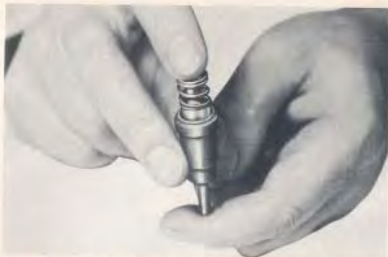
Fig. 43—Place a Finger Over the End of the Oil Inlet Tube, Depress the Plunger and Release It Quickly.
