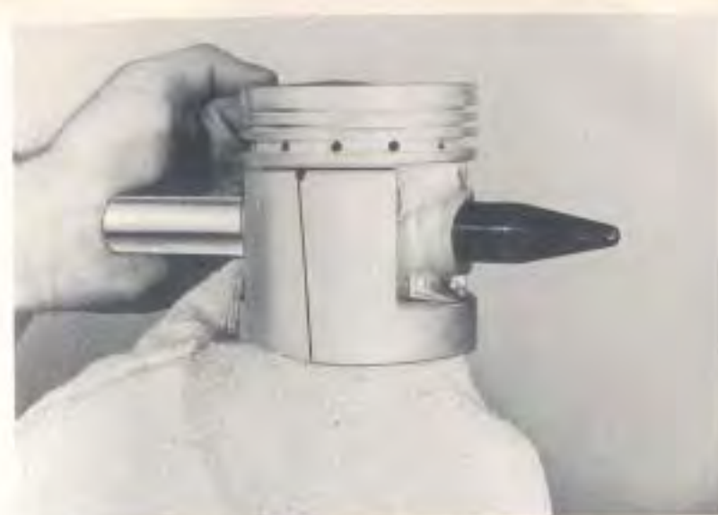
Fig. 23—Place the Piston Pin on the Assembly Pilot and Push into Place as Shown.
