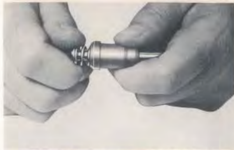
Fig. 39—Twist the Plunger in the Direction That Would "Wind Up" the Spring and Pull Outward.
