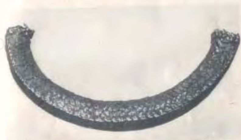
Fig. 28—After the Seal is Formed as Shown, It May Be Fed into Its Groove in the Cylinder Block.
