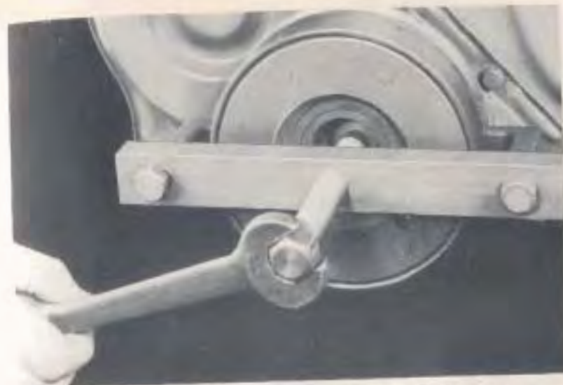
Fig. 30—Vibration Damper Puller J-2582 Is Used to Remove Friction Disc Type Dampers.
