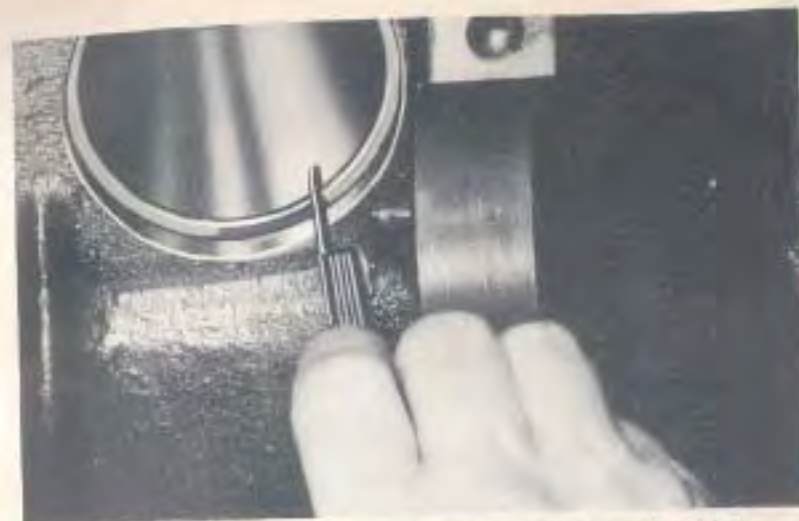
Fig. 15—Checking Piston Ring Gap. Ring Gap Should Be Checked at the Bottom or Unworn Part of the Cylinder.
