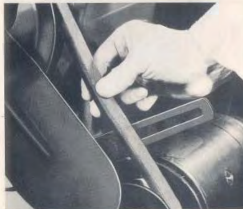
Fig. 52—The Fan Belt Is Properly Adjusted When It Can Be Depressed from \frac{1}{4} Inch to \frac{1}{2} Inch as Shown.
