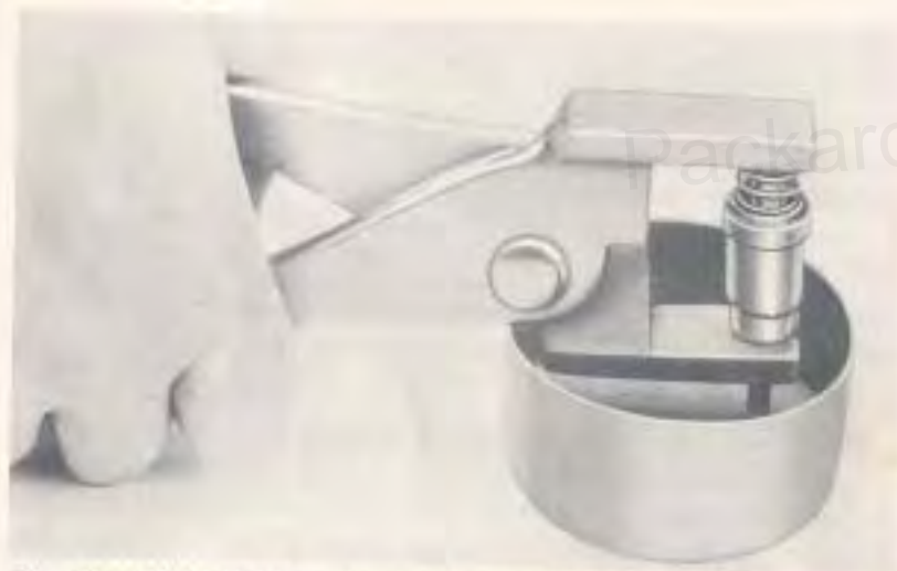
Fig. 41—While Holding the Ball Check Valve Off Its Seat, Depress and Release the Plunger Four or Five Times.
