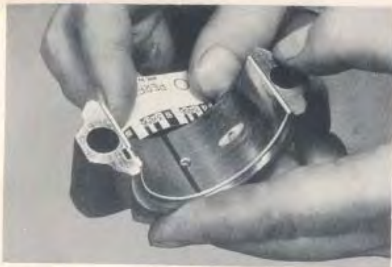
Fig. 26—Compare the Width of the Flattened Plastigage at its Widest Point with the Scale on the Envelope.
