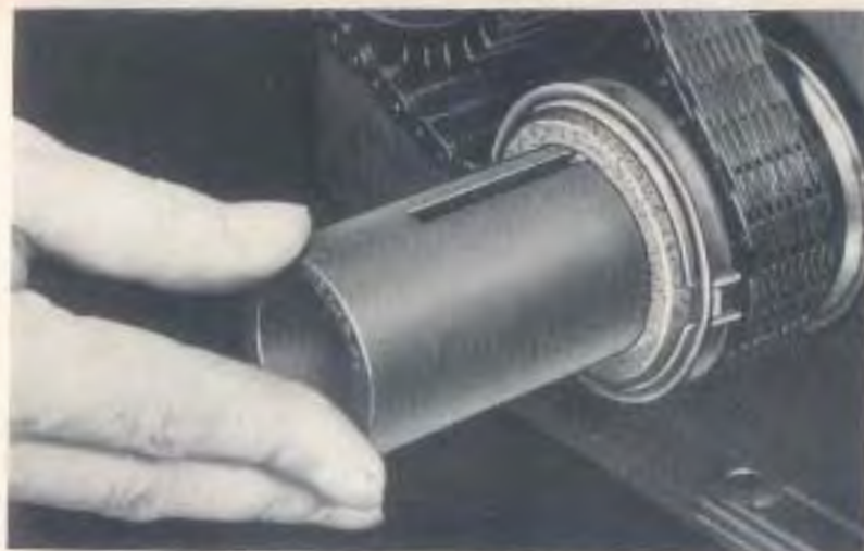
Fig. 32—Gear Cover Aligning Arbor J-2572 Should Be Used When Replacing a Crankshaft Front Oil Seal.
