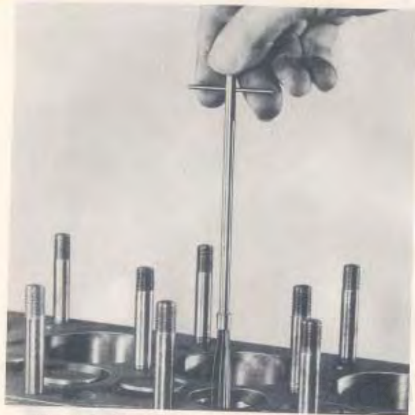
Fig. 35—Valve Guides May Be Cleaned with the Valve Guide Cleaner KMO-122 as Shown.
