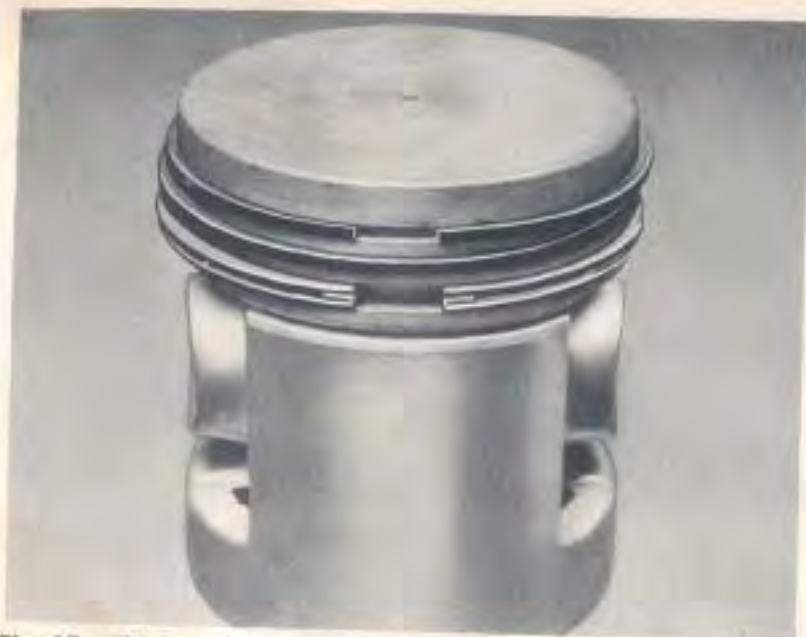
Fig. 17—The Top Compression Ring and the Oil Ring Are Installed with the Gaps Opposite Slotted Side of Piston.
