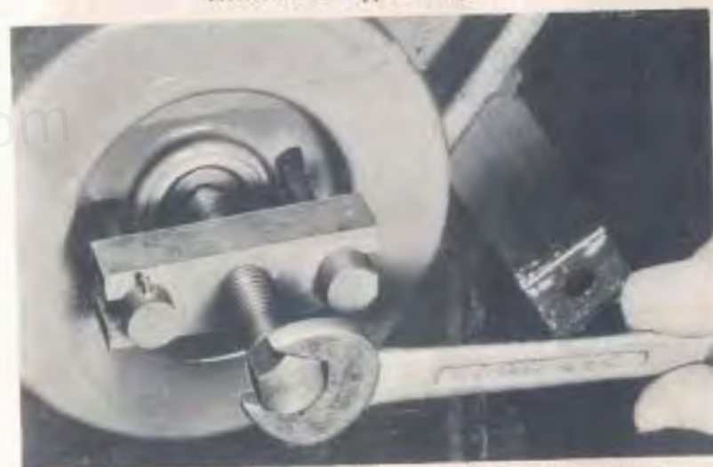
Fig. 31—Vibration Damper Puller J-2636 Is Used to Remove Fluid Suspension Type Dampers.
