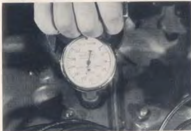
Fig. 54—Check the Compression of Each Cylinder Using a Suitable Gauge and all Spark Plugs Removed.
