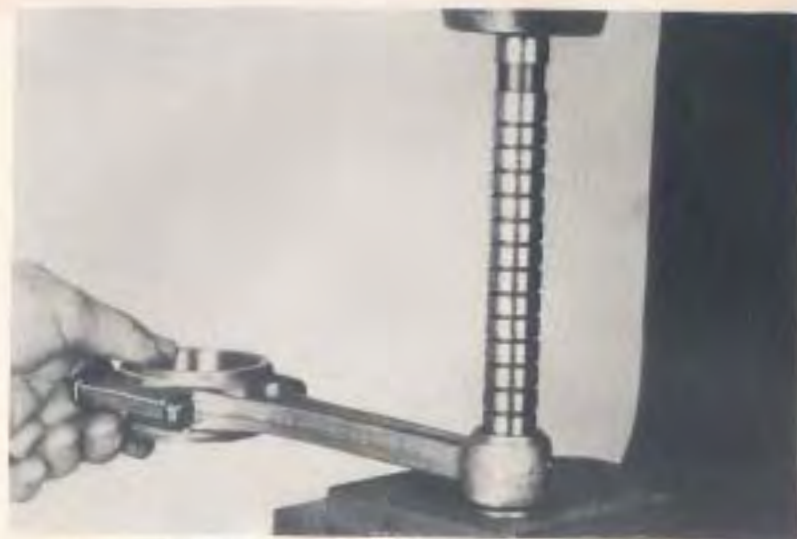
Fig. 19—The Split Type Piston Pin Bushings Should Be Burnished Separately and from the Inside as Shown.
