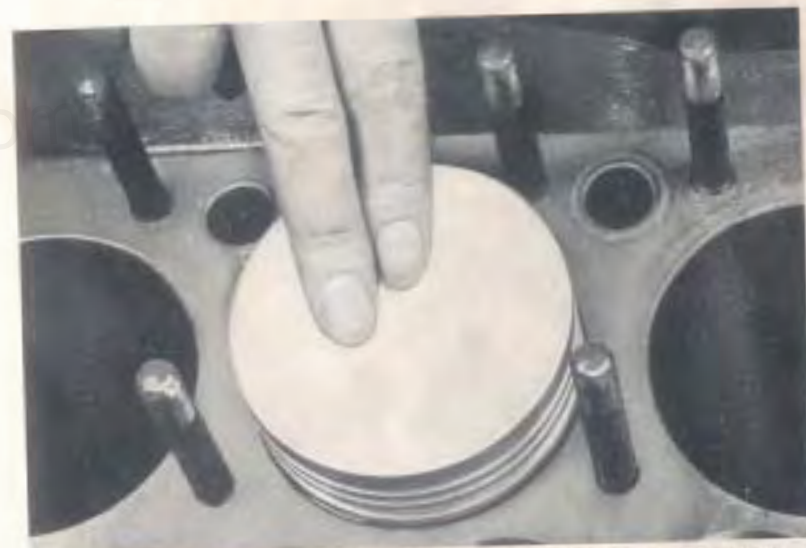
Fig. 13—Piston Fit in Rebored Cylinders Should Be Checked by Applying Pressure with Two Fingers as Shown.
