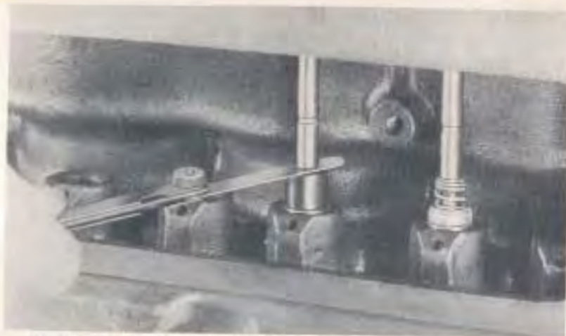
Fig. 38—While Holding the Valve Down on Its Seat, Check the Clearance Between the Valve Stem and the Plug Gauge.
