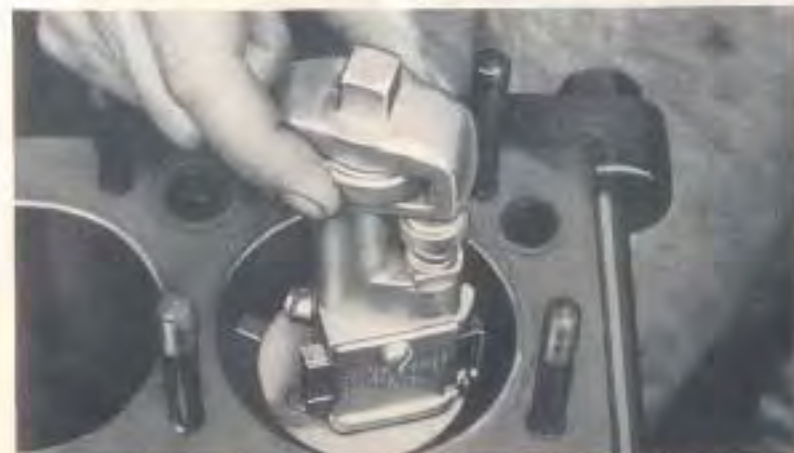
Fig. 6—Turn Large Knurled Knob Clockwise Until Jaws of Centering Head Support the Weight of the Tool.
