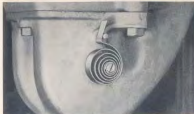
Fig. 51—The Spring Thermostat Should Hold the Counterweight Firmly in the Up Position When the Manifold Is Cold.
