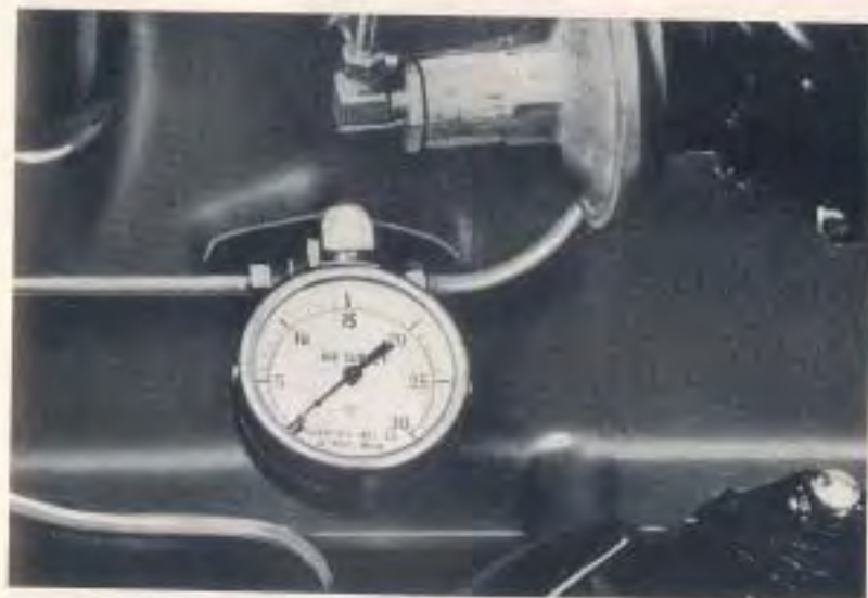
Fig. 44—A Direct Reading Pressure Gauge Installed in Place of the Sending Unit to Check Oil Pressure.
