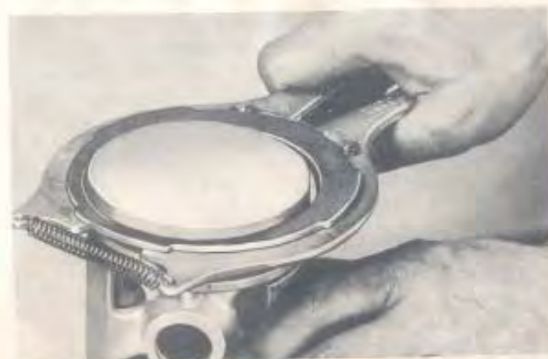
Fig. 16—A Piston Ring Expander Should Be Used to Prevent Over-Expanding or Twisting the Rings.
