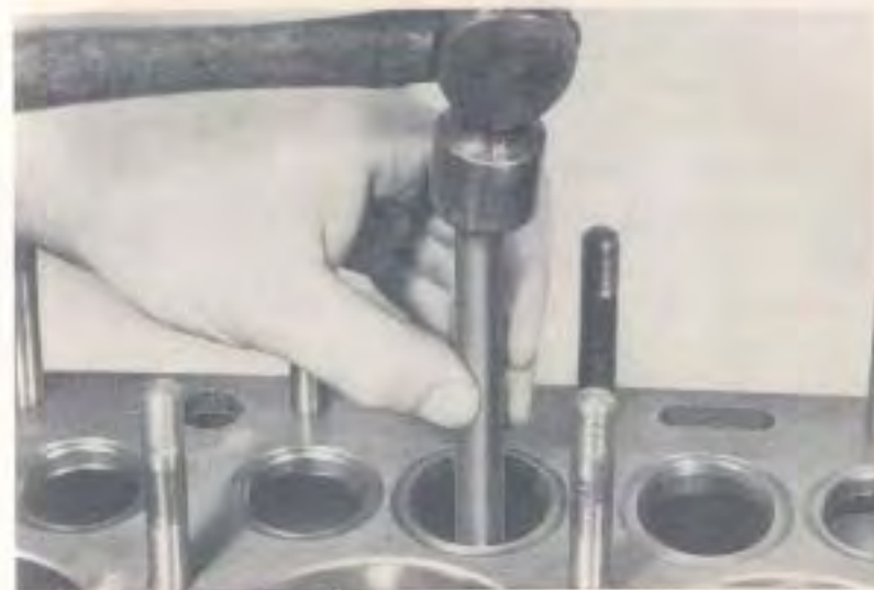
Fig. 36—Drive the Valve Guide Downward with Valve Guide Remover J-2580 as Shown.
