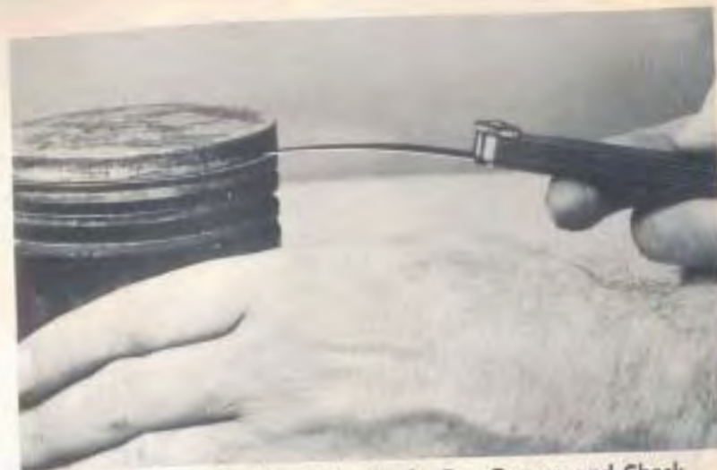
Fig. 12—Install a New Ring in the Top Groove and Check the Clearance Between the Ring and the Top Land.
