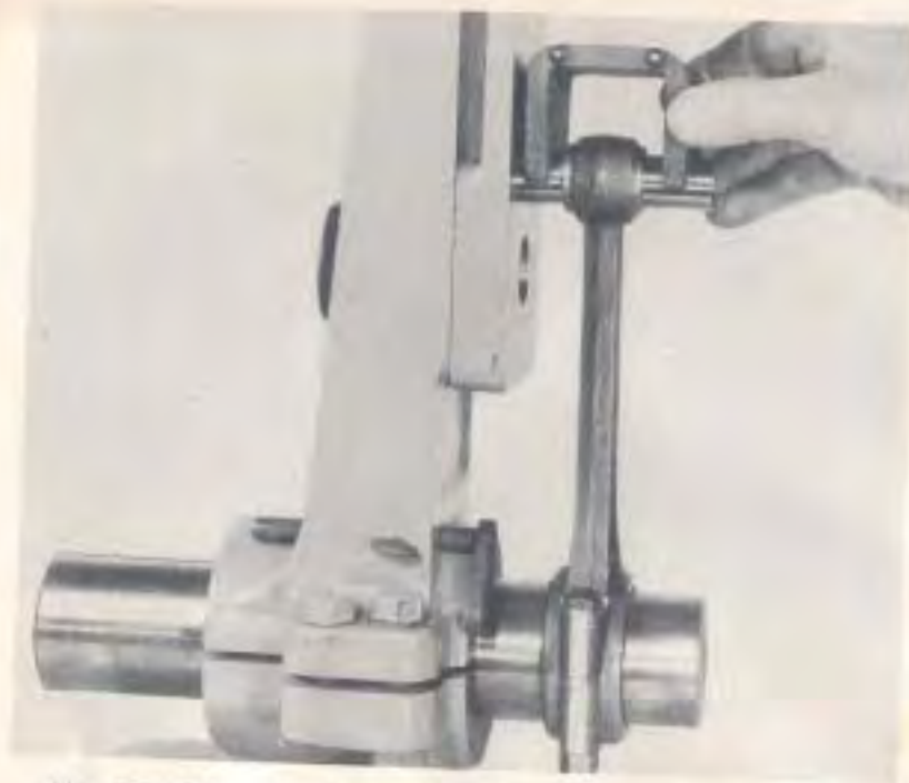
Fig. 22—Using the Connecting Rod Aligning Jig J-874-PA to Check Rod Alignment.
