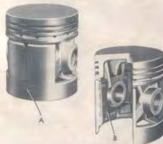
Fig. 4—Packard Piston. Slot "A" Compensates for Skirt Expansion. Strut "B" Thermostatically Controls Expansion.
