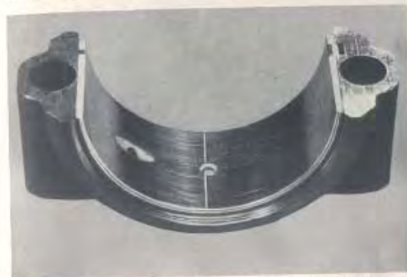
Fig. 25—Place a Strip of Plastigage Across the Full Width of the Bearing Shell as Shown.
