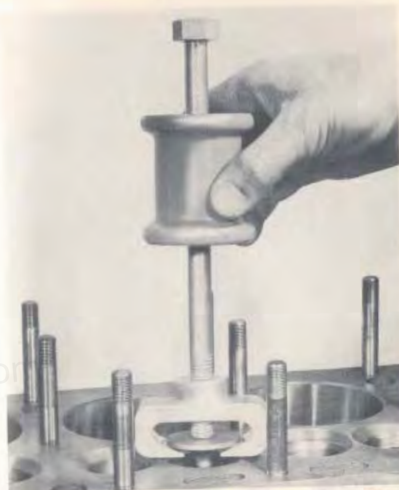
Fig. 34—Tight Valve Remover J-2153 Will Facilitate Removal When Valves Have a Carbon, Gum, or Rust Build-Up.
