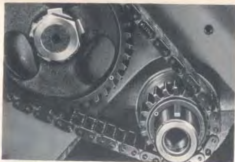
Fig. 46—Crankshaft Sprocket and Camshaft Sprocket Are Properly Related When the "O" Marks Are in Position Shown.
