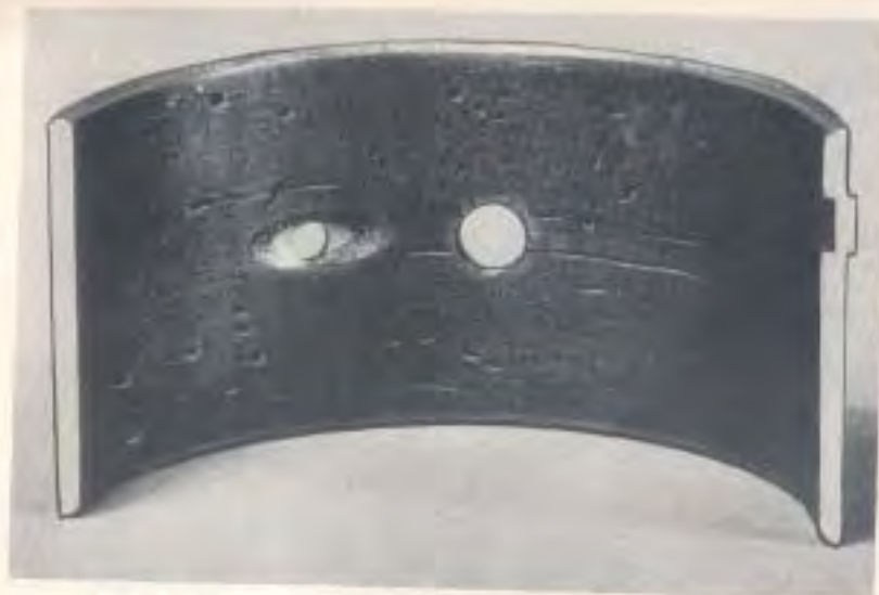
Fig. 24—The Intricate Pattern of Tiny Surface Cracks Is Characteristic of This Type Bearing Shell After Use.
