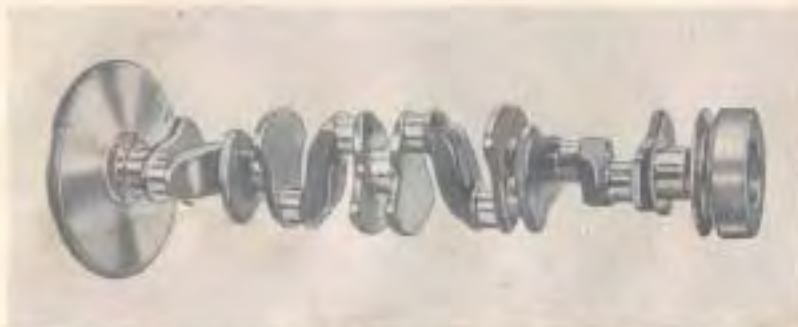
Fig. 2—Packard Eight Crankshaft with Flywheel and Vibration Damper Attached.
