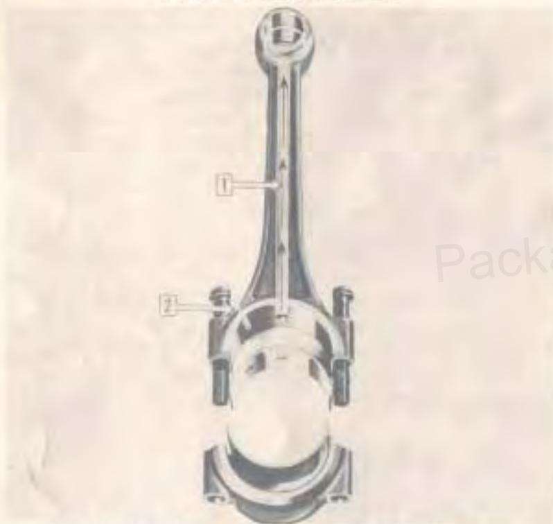
Fig. 3—Exploded View of Connecting Rod and Bearing Assembly. Note the Drilled Oil Passages.
