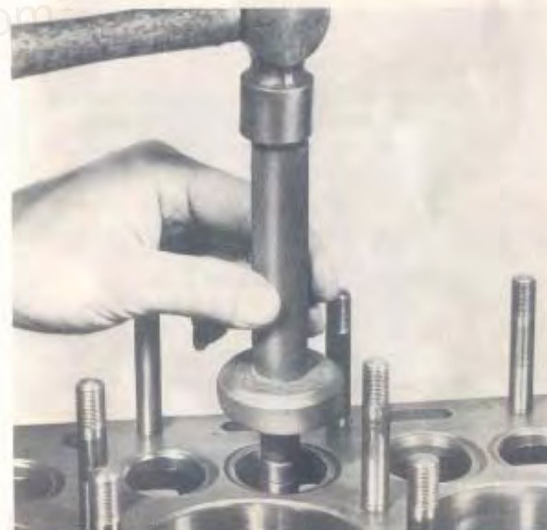
Fig. 37—Both the Inlet and the Exhaust Valve Guides Can Be Driven to Their Proper Depth with the Tool Shown.
