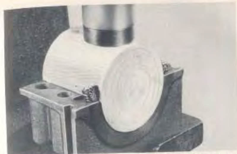
Fig. 27—Pressing the Rear Main Bearing Oil Seal into the Bearing Cap Using an Arbor Press.
