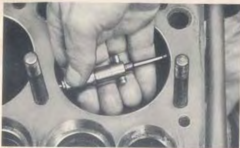
Fig. 10—Measure the Cylinder Wall and Record the Measurement Found at the Point of Greatest Wear.
